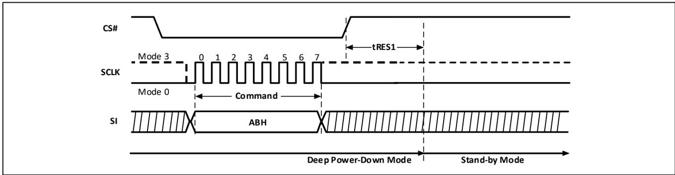
Figure-23. Read Electronic Signature (RES) Sequence Diagram
