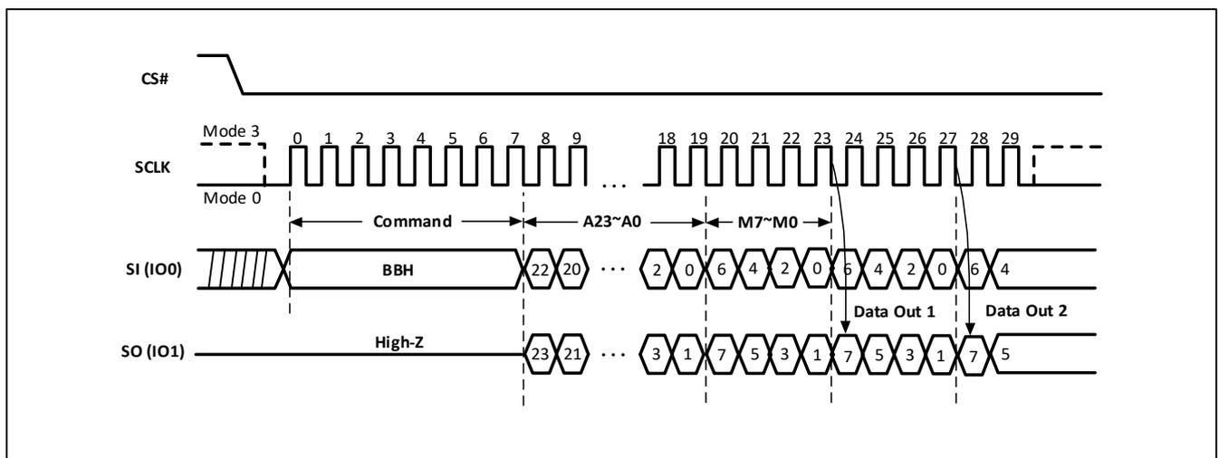
**9.10 Dual I/O Fast Read with “Continuous Read Mode” (BBH)**
