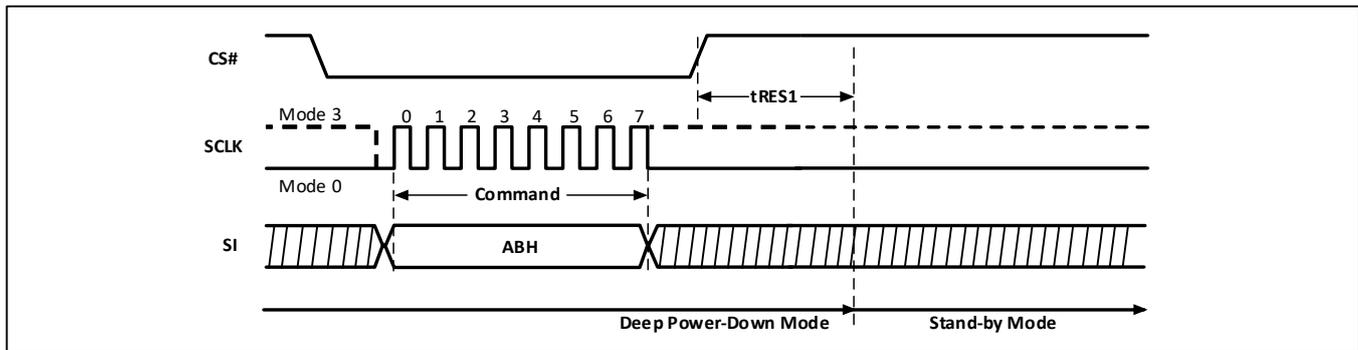
**Figure-24. Read Electronic Signature (RES) Sequence Diagram**
