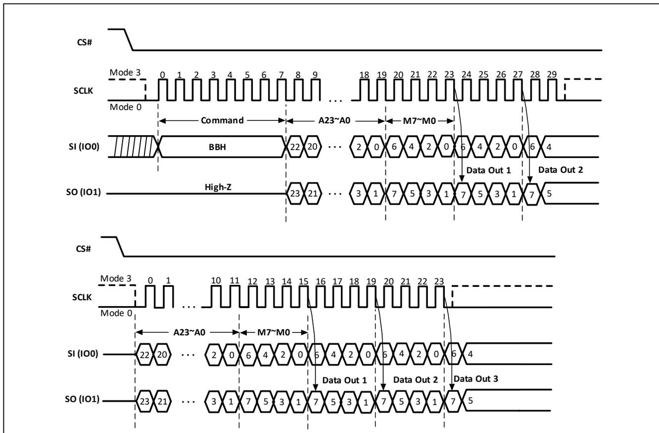
**Note:** Dual I/O Fast Read with “Continuous Read Mode”, if (M5-4)=(1,0). If not using “Continuous Read Mode” recommend setting (M5-4)≠(1,0).
